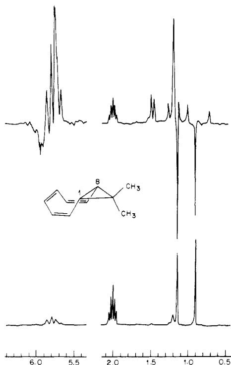
Figure 2. ^1\text{H} NMR spectra (90 MHz) of an acetone- d_6 solution containing 0.02 M each of chloranil and 9,9-dimethylbicyclo[6.1.0]nonatriene ( 1b ) in the dark (bottom) and during UV irradiation (top).
